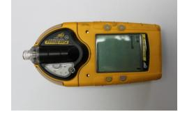
Any location where the concentration is above 50% of the LFL for any part of the test is deemed to be potentially
