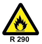
It is recommended that an additional label is fixed to the system to provide basic safety information to service engineers. An example label for an R290 system is shown below.
